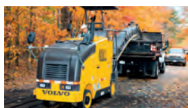
Asphalt milling machines
