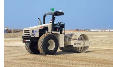
Soil and asphalt compactors
