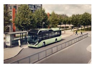
by 60% and carbon dioxide by up to 75%, compared to a conventional Euro 5 diesel bus. It runs in electric mode in average 70% of the route and offers flexibility in operation; it can run as an electric bus in selected areas, but performs as a hybrid on any route. Charging at end stations takes six minutes.
